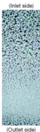
SEM photo of a cross-section of the PSE membrane
